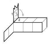
**4a** Variation of step 4 for piece 4, 6 and 7: Let a loop stick out on the underside.
