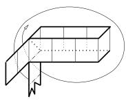
**3a** Variation of step 3 for piece 3, 4, 6 and 7: Pull the tape through under the frame on the right, lay it over the frame on the left.
