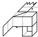
3 Pull the tape through on the top and on the bottom under the vertical frame, let a loop stick out in front (as indicated by the dotted lines).
